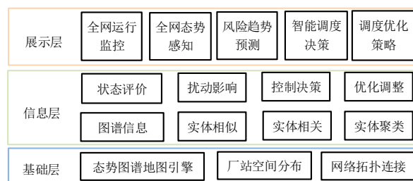
Fig. 13 Functional framework of operation situation knowledge graph visualization engine
